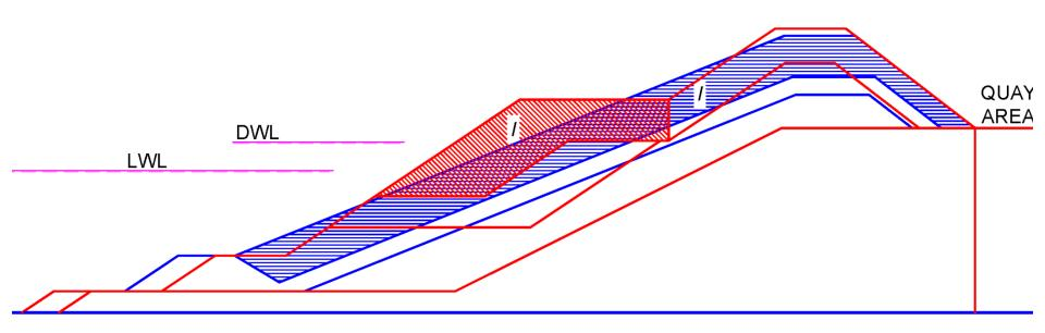
Conventional: two times more 6-10 t rock Total volume of rock similar Berm breakwater: construction by excavator only
