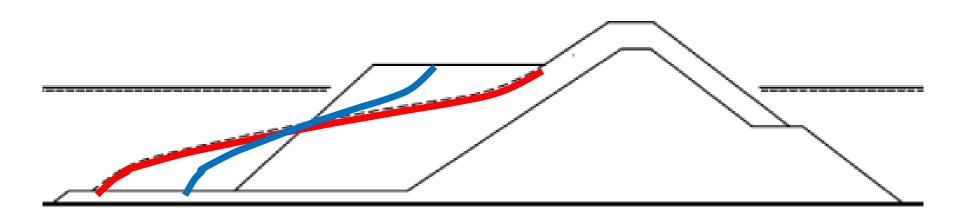
Fully reshaping berm breakwater (mass armoured)
