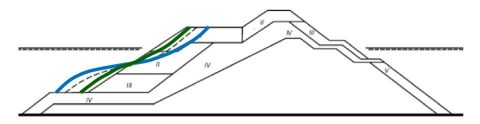
Partly reshaping Icelandic-type berm breakwater
