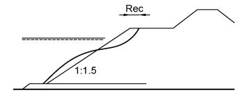
Berm level and width High berm less recession Large berm width reduces recession
